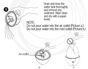
Please read the instructions carefully before using. Manufacturer accepts no liability for damage caused by incorrect use of the NOW® Solutions Ultrasonic
