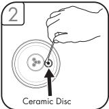
Wipe base with soft damp cloth. Using a cotton swab with warm water or alcohol, gently clean the ceramic disc to remove excessive oil residue.
