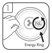
First disconnect the power. Unlock the energy ring.
